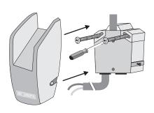
Attach the sensor to the wall. Replace front cover and secure with screws provided
