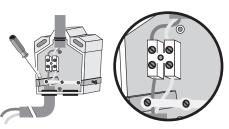
**TRANSFORMER** 3. Connect the cable leads to the terminals
