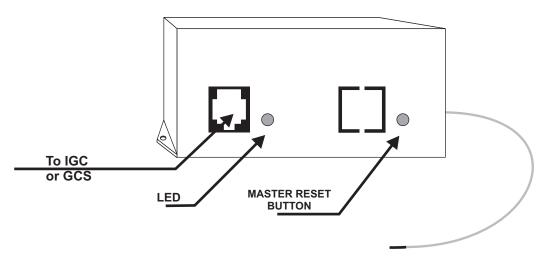
IGC RECEIVER: Part No.: 1810481 GCS RECEIVER: Part No.: 1810854
