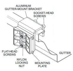
Securely attach rain sensor mounting plate to aluminum gutter mount bracket using flat head screws and nylon locking nuts. Slide gutter mount bracket over gutter lip and secure with socket-head screws.
