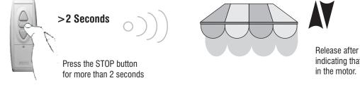
Release after the awning jogs briefly UP/DOWN indicating that the change has been memorized in the motor.
